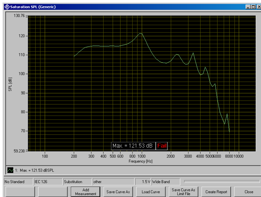
Fig. 29 Display window of saturation sound pressure level measurement
