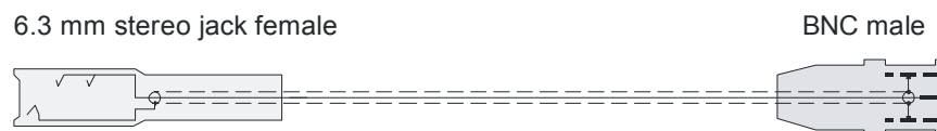
Fig. 3 Adapter cable to connect the R&S UPL-B7 battery supply cable to the “ANLG AUX OUT” of the R&S UPV
