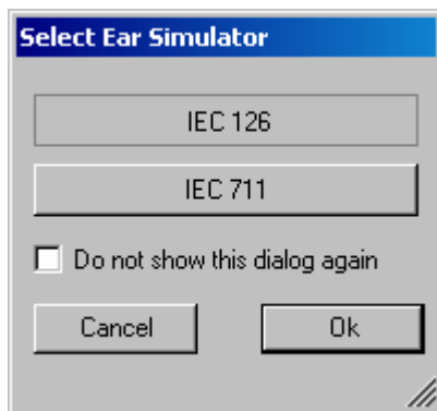
Fig. 5 Query window for selection of ear simulator
